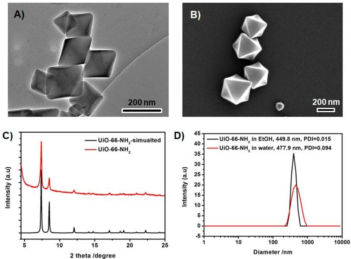
**Fig. S12.** TEM (A) and SEM (B) image of UiO66-NH<sub>2</sub> MOF NPs. (C) Wide PXR patterns of the simulated UiO66-NH<sub>2</sub>, and as-synthesized UiO66-NH<sub>2</sub>. (D) DLS data of the as-synthesized UiO66-NH<sub>2</sub> in water or EtOH.
