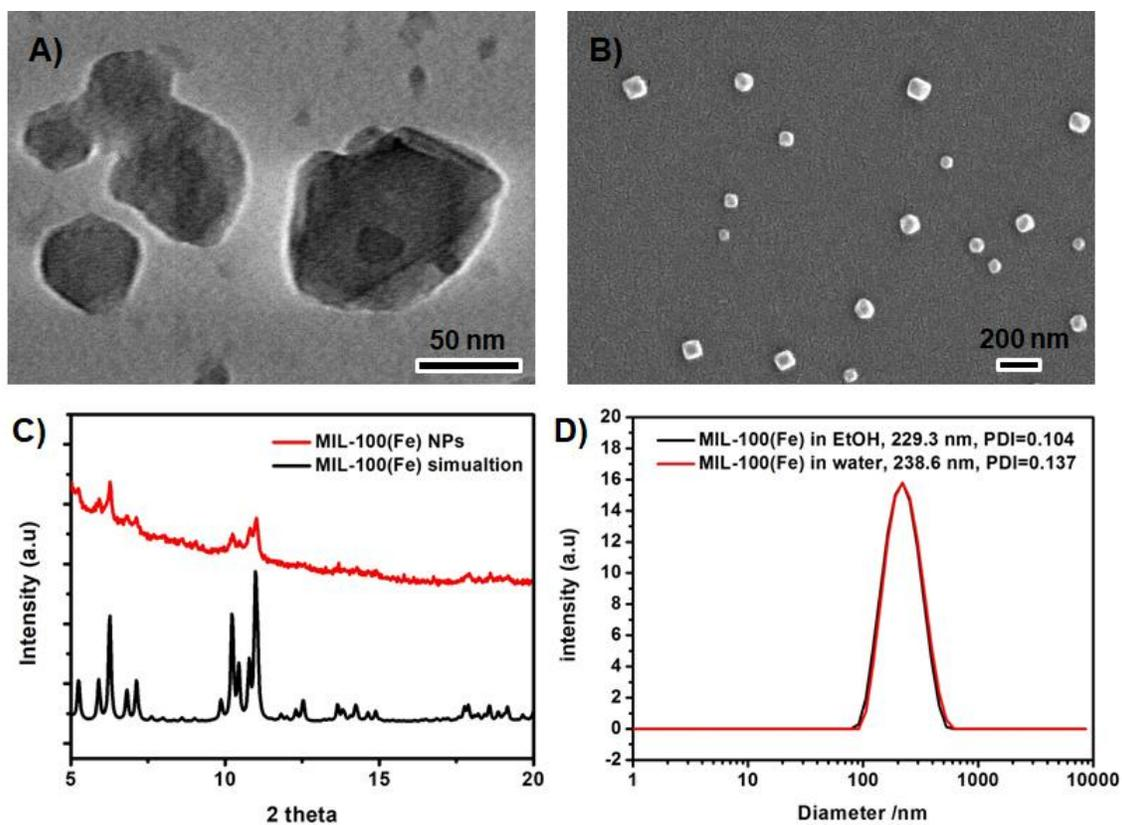
**Fig. S11.** TEM (A) and SEM image (B) of MIL-100(Fe) NPs. (C) Wide PXRD patterns of the simulated MIL-100(Fe), and as-synthesized MIL-100(Fe). (D) DLS data of the as-synthesized MIL-100(Fe) NPs in water or EtOH.
