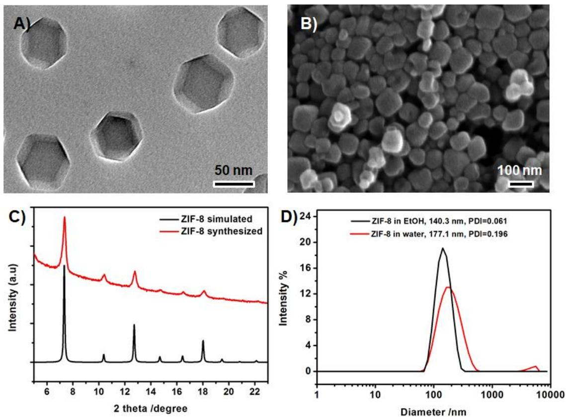
**Fig. S10.** TEM (A) and SEM image (B) of ZIF-8 NPs. (C) Wide PXRD patterns of the simulated ZIF-8, and as-synthesized ZIF-8. (D) DLS data of the as-synthesized ZIF-8 NPs in water or EtOH.
