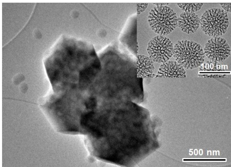
**Fig. S7.** TEM image of the NP of MSN@ZIF-8; insert is the TEM image of MSN.
