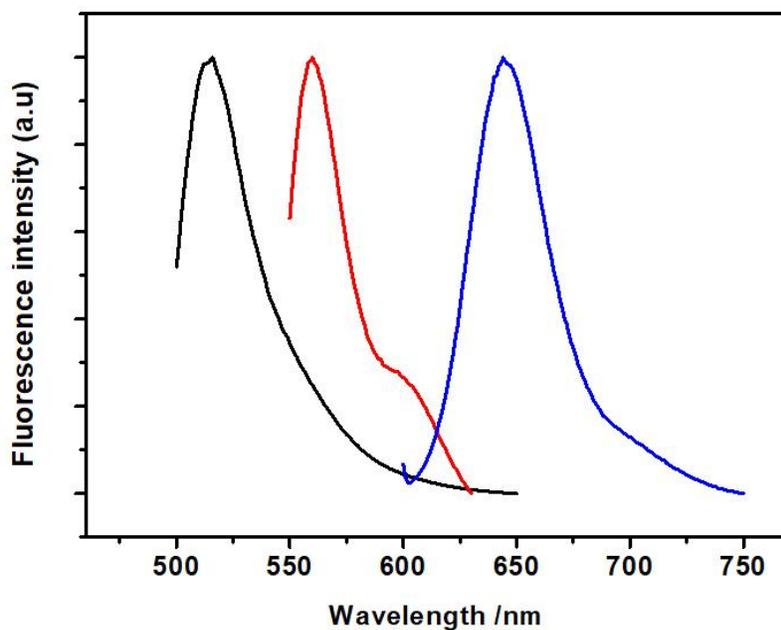
**Fig. S37.** Fluorescent emission spectra of mesoporous silica NPs functionalized with different fluorescent dyes.
