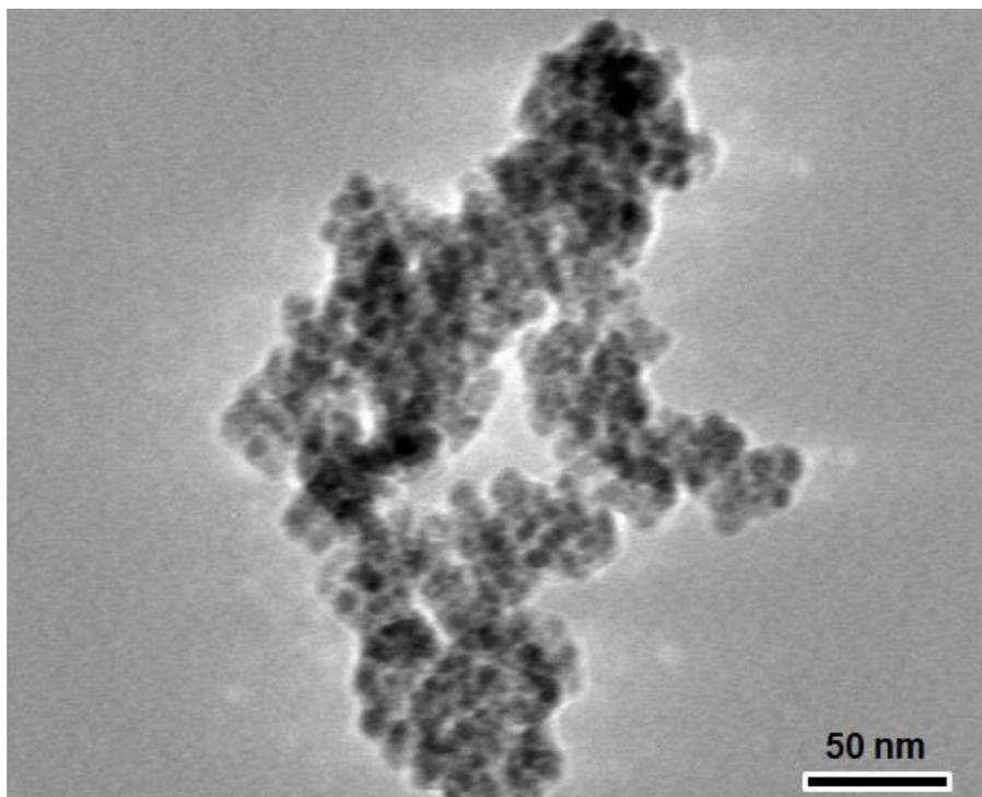
**Fig. S14.** TEM image of  $\text{Fe}_3\text{O}_4$  NPs
