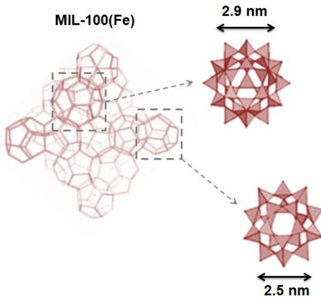
**Fig. S35.** Schematic illustration of the two mesocages in MIL-100(Fe)
