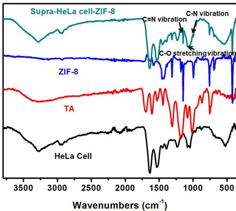
**Fig. S2.** Fourier transform infrared spectrophotometry (FT-IR) of native HeLa cells, tannic acid, ZIF-8 NPs, and Supra-HeLa cell-ZIF-8.
