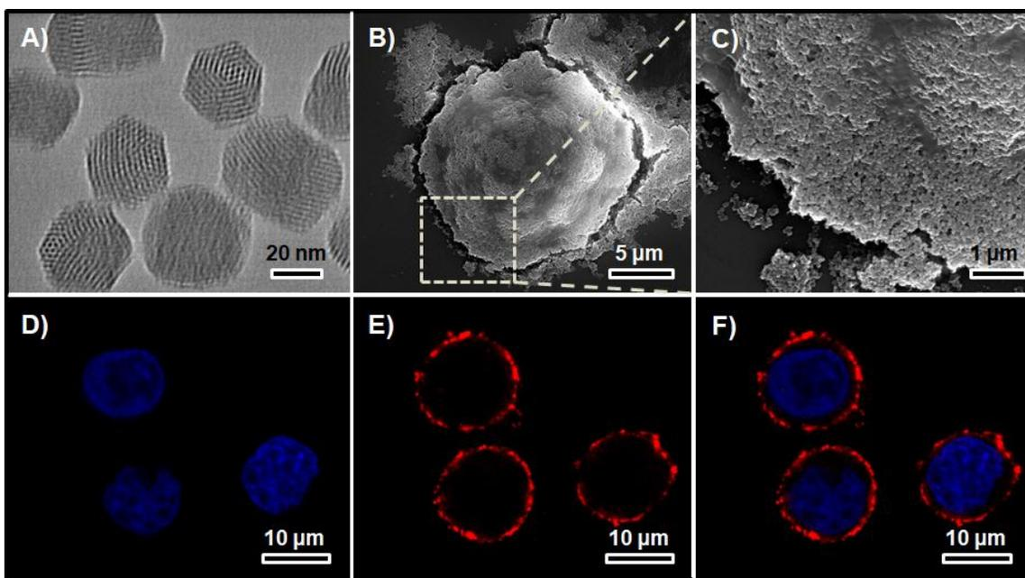
**Fig. S17.** (A) TEM image tannic-modified mesoporous silica NPs. (B-C) SEM image of Supra-HeLa cell-mSiO<sub>2</sub>. (D-F) Fluorescence image of Supra-HeLa cell-mSiO<sub>2</sub>: nucleus, mSiO<sub>2</sub> exoskeleton, combined image (from left to right).
