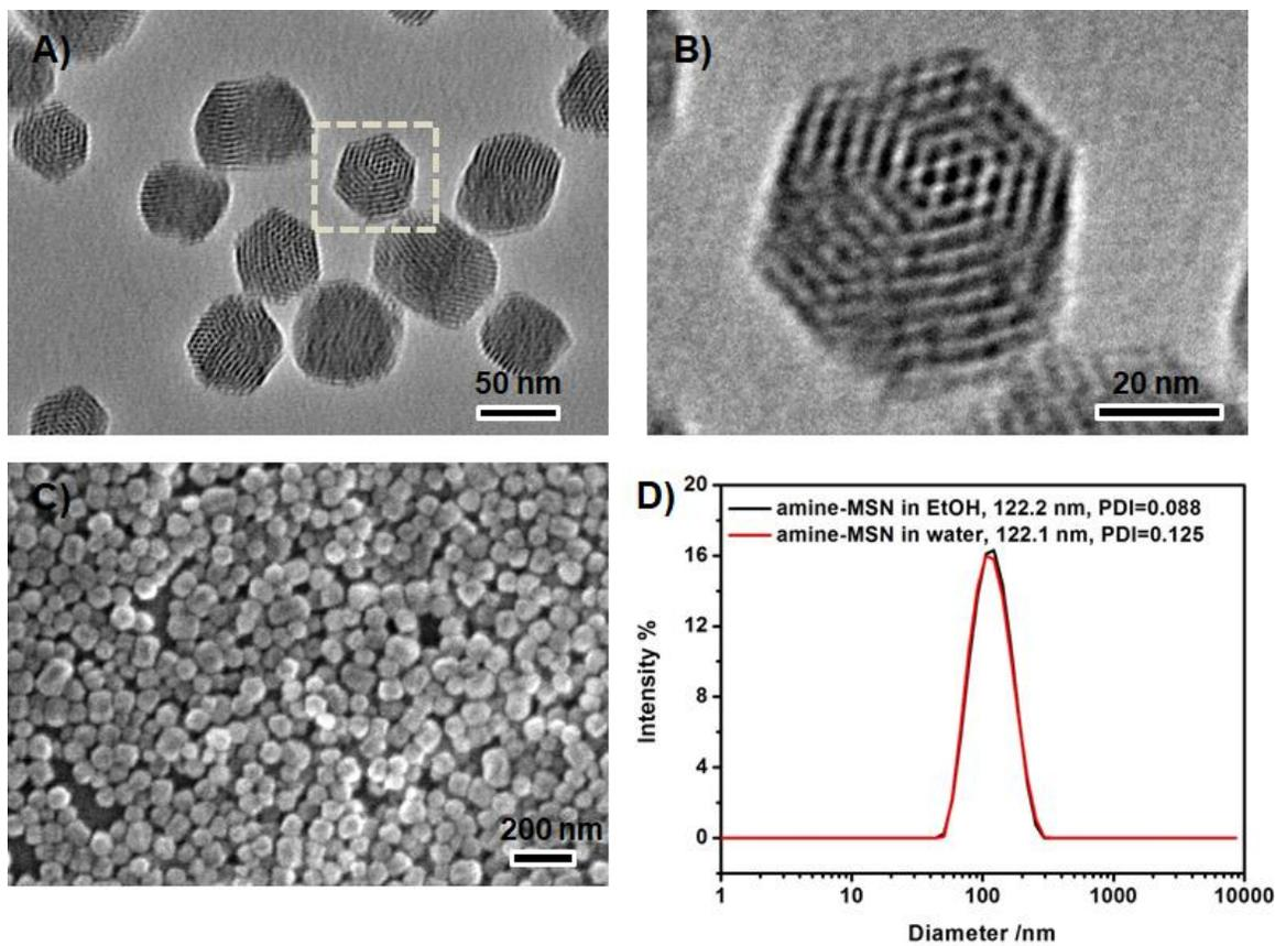
**Fig. S13.** TEM (A-B) and SEM (C) images of amine-functionalized mesoporous silica NPs; DLS data of amine-functionalized mesoporous silica NPs in water or EtOH.
