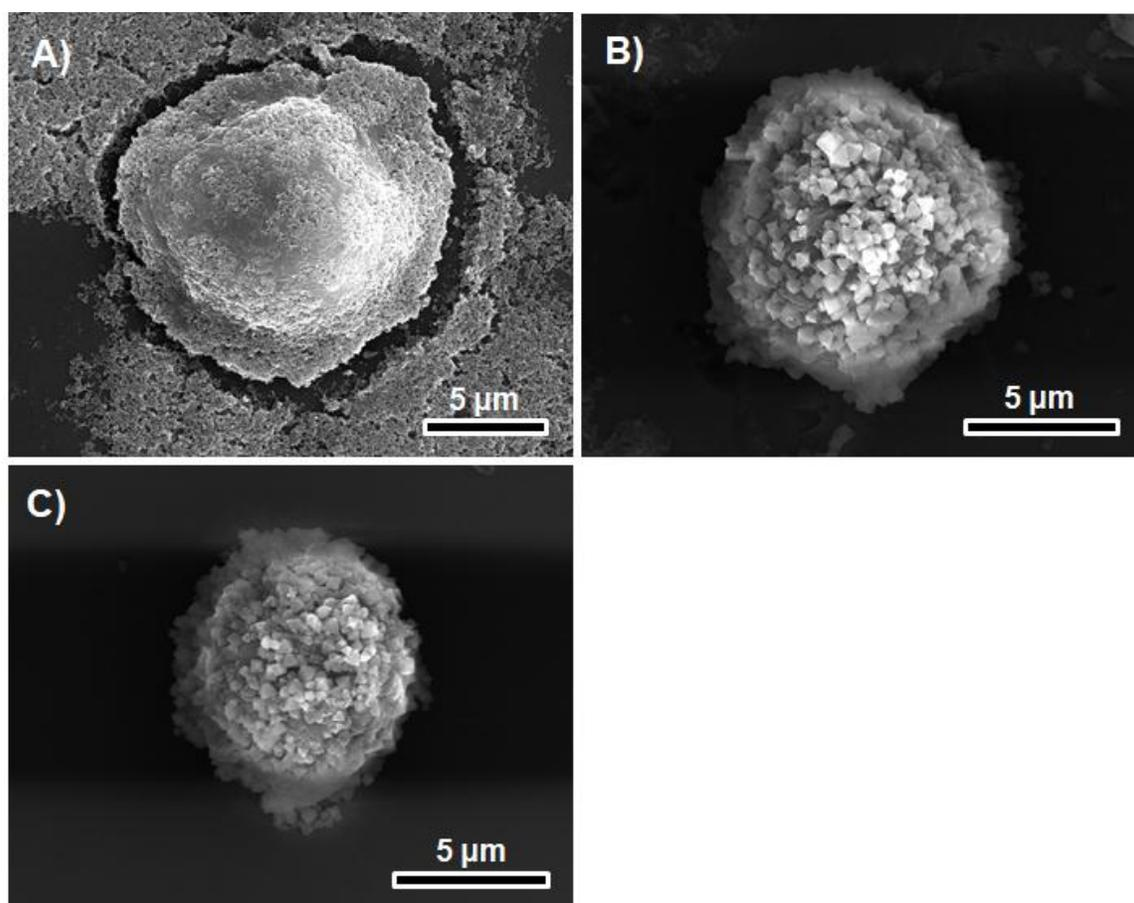
**Fig. S16.** SEM images of the Supra-HeLa cell-MIL-100 (Fe) (A), Supra- Raw 264.7 cell-UiO-66-NH<sub>2</sub> (B), and Supra-HeLa cell-MET-3(Fe) (C).
