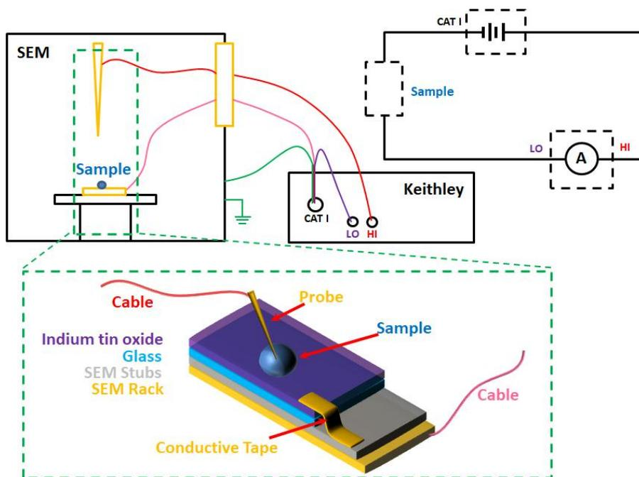
**Fig. S40.** Schematic illustration of in-situ SEM electrical characterization.
