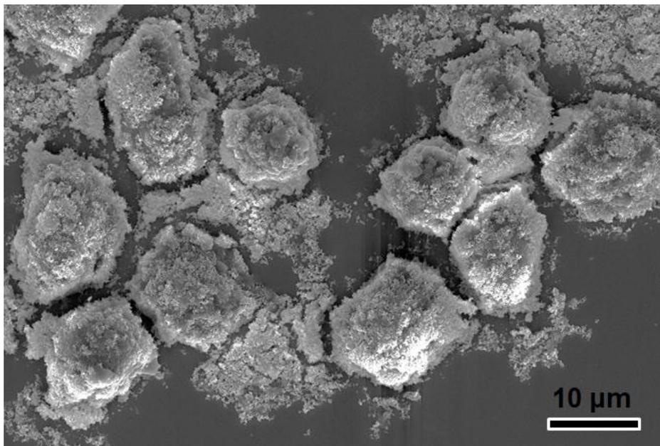
**Fig. S3.** SEM image of a Supra-HeLa cell-ZIF-8.
