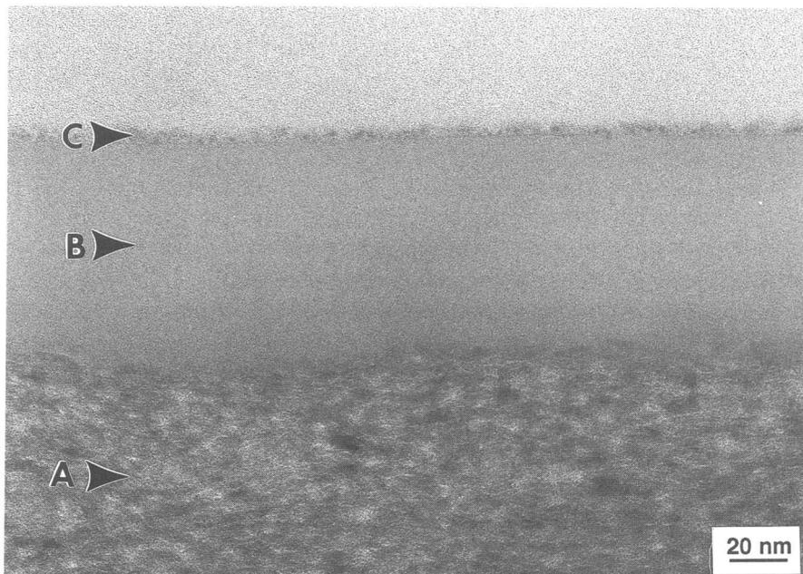
Fig. 8. Cross-sectional TEM image of rhodium particles attached to surface of porous SiO<sub>2</sub> layer on  $\gamma$ -Al<sub>2</sub>O<sub>3</sub> membrane support prepared by the silylation-[(1,5-COD) RhCl]<sub>2</sub> reaction approach. Region A indicates  $\gamma$ -Al<sub>2</sub>O<sub>3</sub> support layer, B indicates porous SiO<sub>2</sub> layer, and C indicates layer of rhodium particles.
