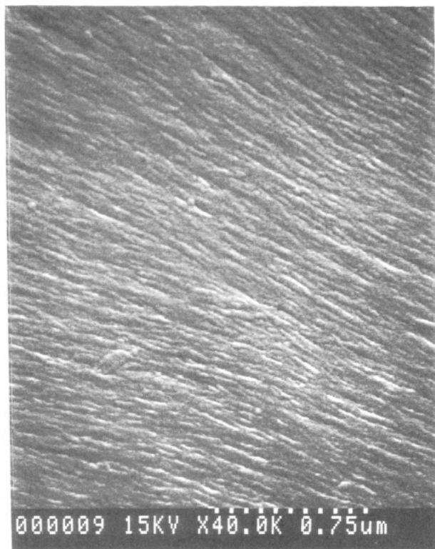
Figure 3. SEM micrograph of 100% Si synthetic imogolite showing the long range order of the collected material.
