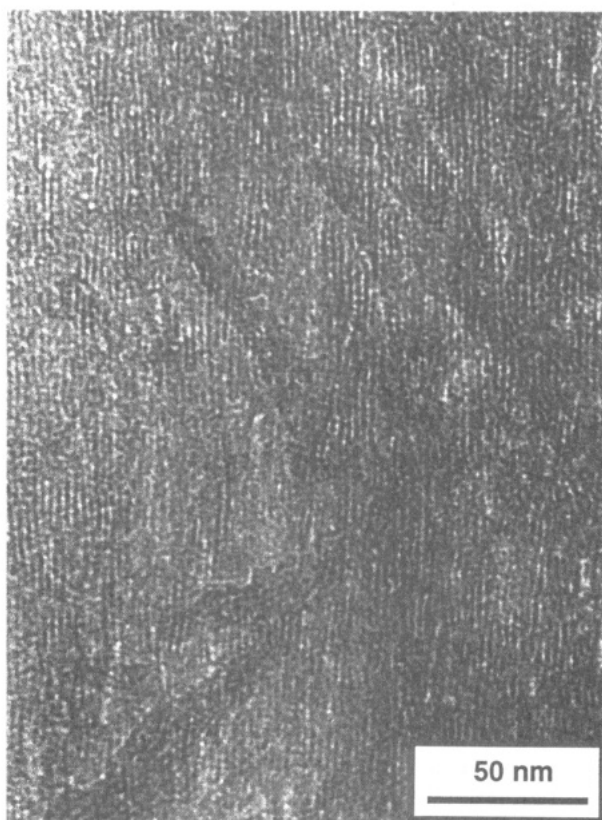
Figure 4. (a, top) TEM micrograph and electron diffraction of 100% Si synthetic imogolite showing local ordering and tube spacing of approximately 2.5 nm. (b, bottom) TEM micrograph of 50% Si synthetic imogolite showing local ordering and tube spacing of approximately 2.5 nm.
