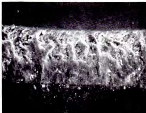
Figure 4. Section of glass 60-4 after heat treatment for 48 days at 375°C (bar = 0.01 mm)
